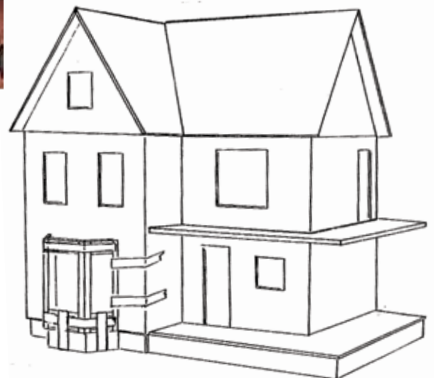
Illustration #5 Glue the Bay Walls Together, to the Bay Base Floor, and to the Foundation
