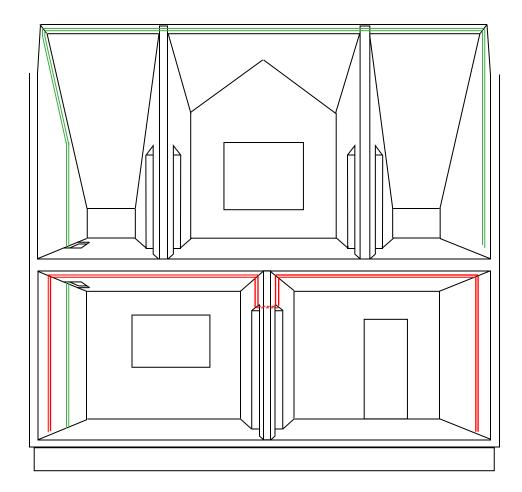
Ceiling Loop if you're wiring using E-Slots: lay the Ceiling Loop lined up with the Main Loop *copper-over-copper* and *blue-over-blue*, with at least 11/2" of overlap.
