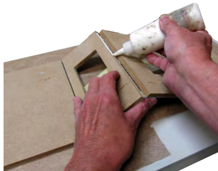
Lift the joints for glue
