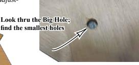
7. Rotate the Bottom Deck (with the 'Big Hole') without letting the Turntable slide on the Upper Deck. Find one of the (4) smallest holes in the Narrow Ring.
