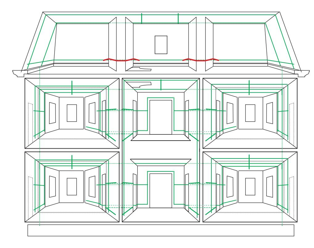
Adding the Attic Partitions later: Install the Attic Partitions and wire them 1/4" higher than the baserun on the Front Roof with 11/2" flaps on the Front Roof. Make sure the copper and blue wires match the copper and blue on the Front Roof run. The Attic Partition Baserun will turn down as it folds to the Front Roof and the extra 1/4" is necessary so the wire colors will line up for the eyelets in a place you can reach with your eyelet tool.
