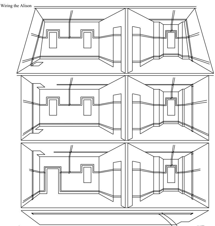
Here's a basic wiring pattern. Modify the exact positioning of the ceiling runs of tapewire based on your interior plan. The Main Loop will start under the Base Floor, go up the stairholes and through the E-slot in the Top Floor stairhole, then up the roof, across the Rooftop, down the roof, and through the E-slots on the other side, back to the underside - all in one piece.
