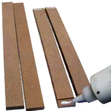
a. Put glue in the grooves
