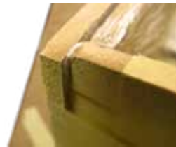
If the Dormer Side sticks out in front, file or trim it now
