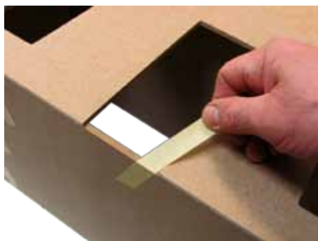
Tape inside the door cutout
