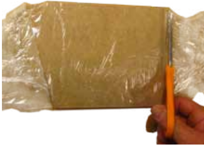
Plastic wrap on the Attic Partition - avoid bunches and wrinkles
